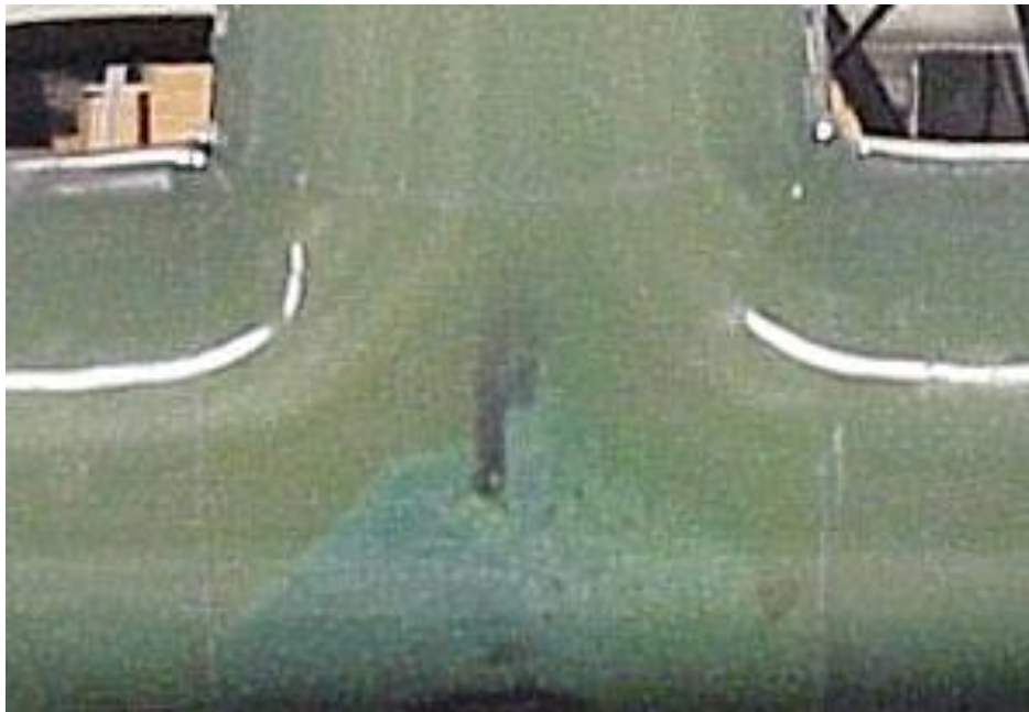
Figure 4.28 Photograph of the solid deposit observed on the electrodes during the EK experimental runs
